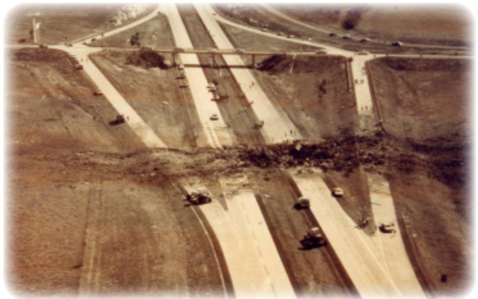
*This photo shows the crater (approximately 75' in diameter and 30' deep) remaining after someone fired a rifle at a tractor-trailer hauling dynamite in 1970.*
